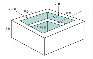
2. How many cubic feet of concrete are needed to build the hot tub?
