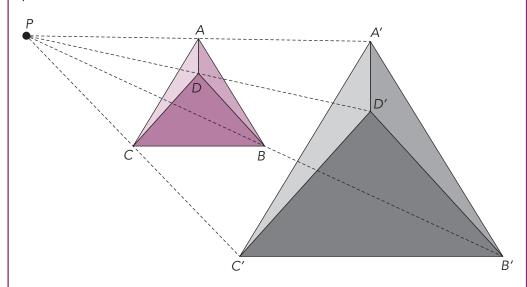
The scale factor can be expressed as  $\frac{PA'}{PA} = \frac{PB'}{PB} = \frac{PC'}{PC} = \frac{PD'}{PD}$ .
